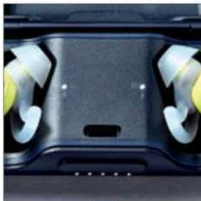
Individual LEDs indicate if each earbud is charging.
