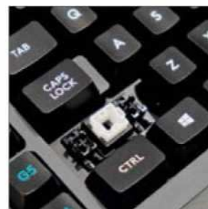
The Romer-G switches use their own key stem design, so they won't work with most third-party keycaps.
