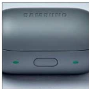
The LEDs glow green or red to indicate charging.
