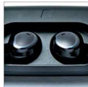
LEDs on the earbuds themselves indicate the battery status.
